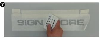
With the application tape still covering the face of the graphic, press the graphic firmly onto the application surface with a squeegee. Press from the center of the graphic to the outside edge using overlapping strokes.
